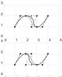
The  $ts\{t\}$  modifier changes the tension of the left and right control points next to the interpolation point which stands in front of the modifier. In the next example a negative tension value leads to a rather surprising effect.
