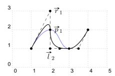
With the  $t\{t\}$  modifier you can change the tension of the automatically computed control points of the current Bezier spline.
