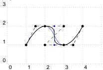
As you can see from the example both control points of the current spline are affected by the  $t\{t\}$  modifier. If you want to change the tension of just the left or right control point you can use the  $t\{t\}$  or  $tr\{t\}$  modifier, respectively, as demonstrated in the following two examples.
